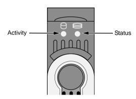
Figure 4. VTrak M500f/i/p disk carrier LEDs
